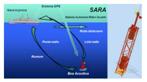
Via a bidirectional RF transmission link, data can be exchanged with the buoy, including the time-history from one of the three connected hydrophone sensors and its spectrum, battery voltage level and GPS position of the buoy.
