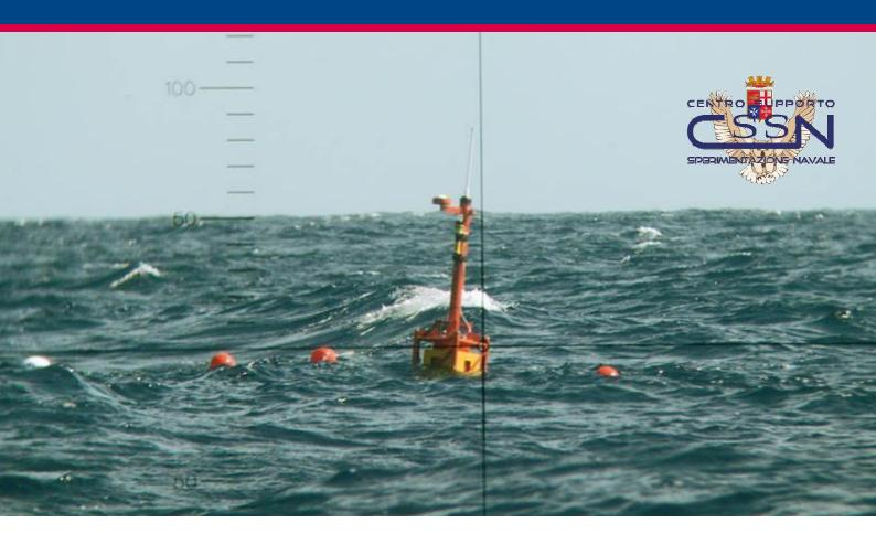
This application note discusses the solution used for the detection of acoustic emissions of surface and underwater vessels by means of the "Autonomous Acoustic Measurement System" (*Sistema Autonomo per Rilievi Acustici*, **SARA**). Activities were carried out by the Italian Navy at the Naval Experimentation and Support Center (*Centro di Supporto e Sperimentazione Navale*, CSSN) of La Spezia.
