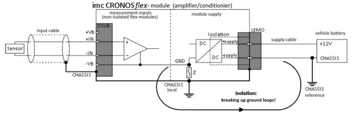
Z describes a high-impedance connection that capacitively short-circuits RF interference.
