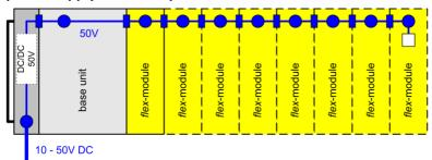
The current-carrying limit on the Module connector also limits the amount of signal conditioning modules which can be stacked directly. The higher the supply voltage is set, the less this limit matters, since the modules' (constant) power consumption leads to correspondingly low currents. The optional supplemental supply unit will convert the 10 V to 50 V input voltage to a fixed intermediate circuit voltage of 50 V at max. 100 W.
