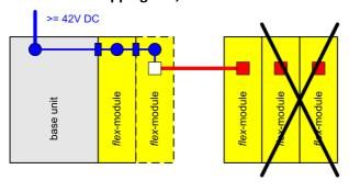
PoEC-supply of one or more modules ensures indirect activation/deactivation through the supplying unit and thus, for example, remote switching by the base unit's main switch.
