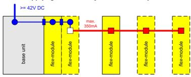
Depending on the power consumption of the module type used, up to three imc CRONOSflex Modules can be powered jointly. The overview table below states the respective power consumption specs.
