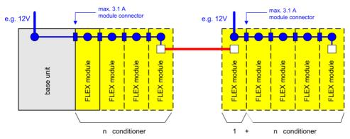
Separately powered individual signal conditioners or conditioner blocks are activated/deactivated by connecting their respective supply voltage. They are not coupled to the base unit's global main switch.
