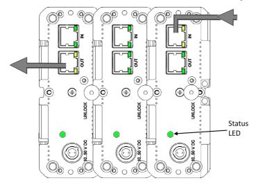
Constant yellow lights on the terminals indicate the system expects connection of an external network or patch cables, where the bus line originating at the base unit is connected at "IN" terminals and the line leading outward to any further bus subscribers is connected to the "OUT" terminal.
