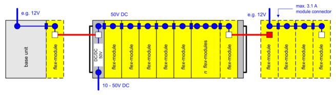
In conjunction with the supplemental power supply, a block only of conditioners can be activated not only by connecting the local power supply, but remote activation can be achieved by means of the connecting network cable. This means that this isolated island of modules can also be switched on/off by the base unit's main switch. However, this only applies to contiguous blocks powered by the supplemental supply.
