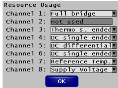
Channel 1: Select the measuring mode for the channel here. The following settings are available in the standard version:
