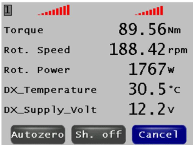
Fig. 111: Power measurement (example image)
