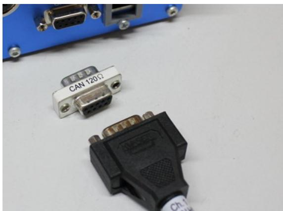
Fig. 57: CAN terminating resistor
