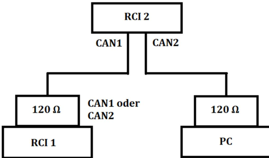
Fig. 59: Example for a CAN network, consisting of 2 D<sup>x</sup>-RCIs and one PC.
