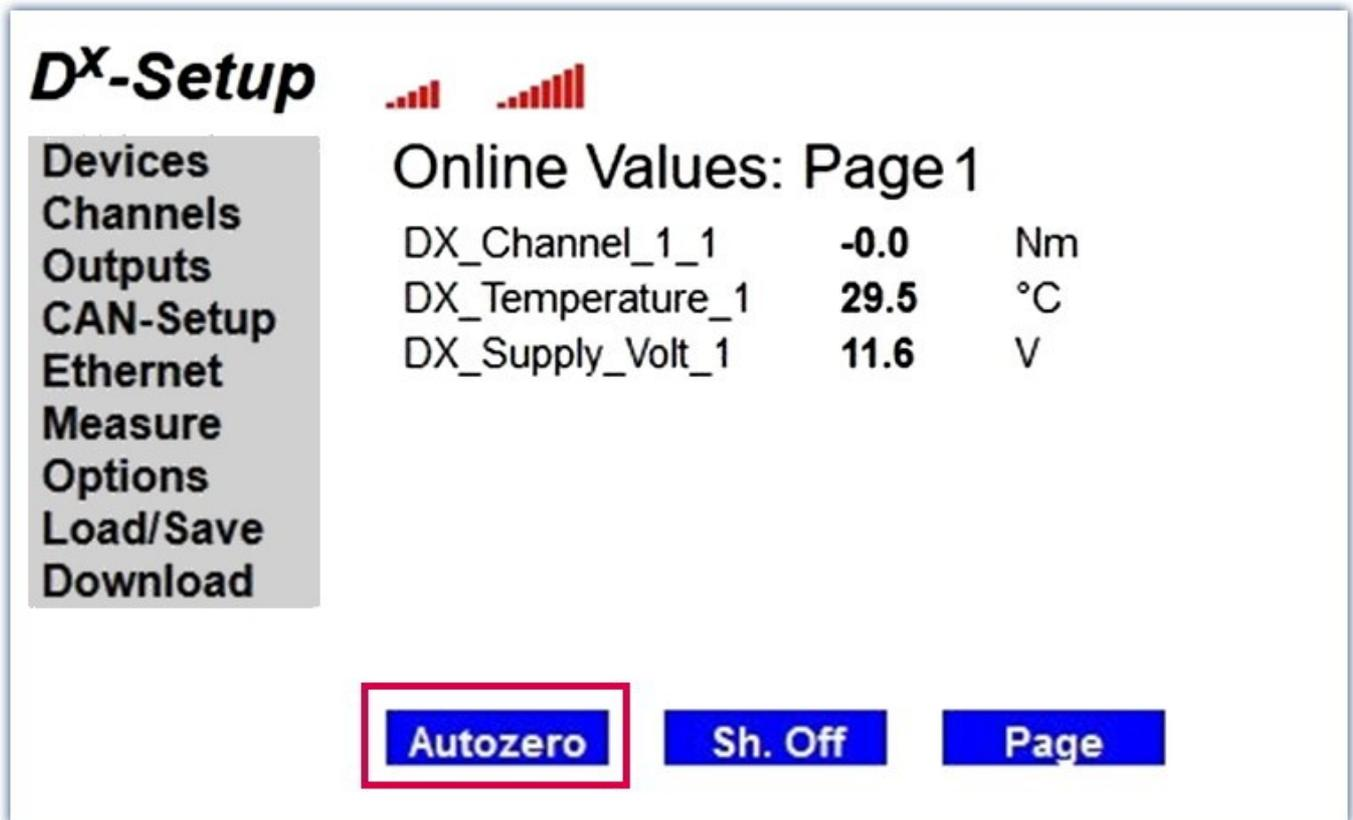
Fig. 89: Trigger Autozero during measurement
