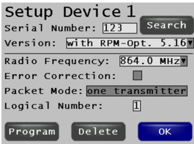
Fig. 105: Version with RPM option
