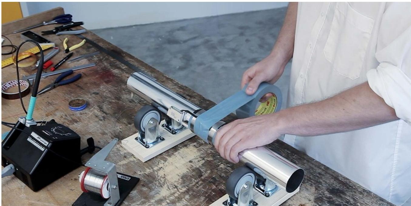
Fig. 42: Apply gray tape for isolation and protection
