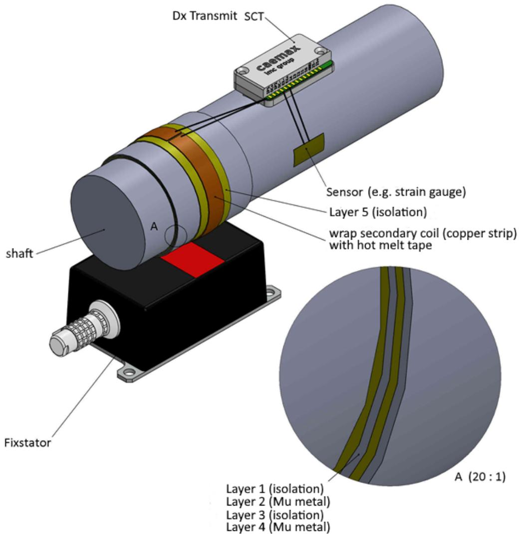
Fig. 19: Overview for an installation of the Fixed stator
