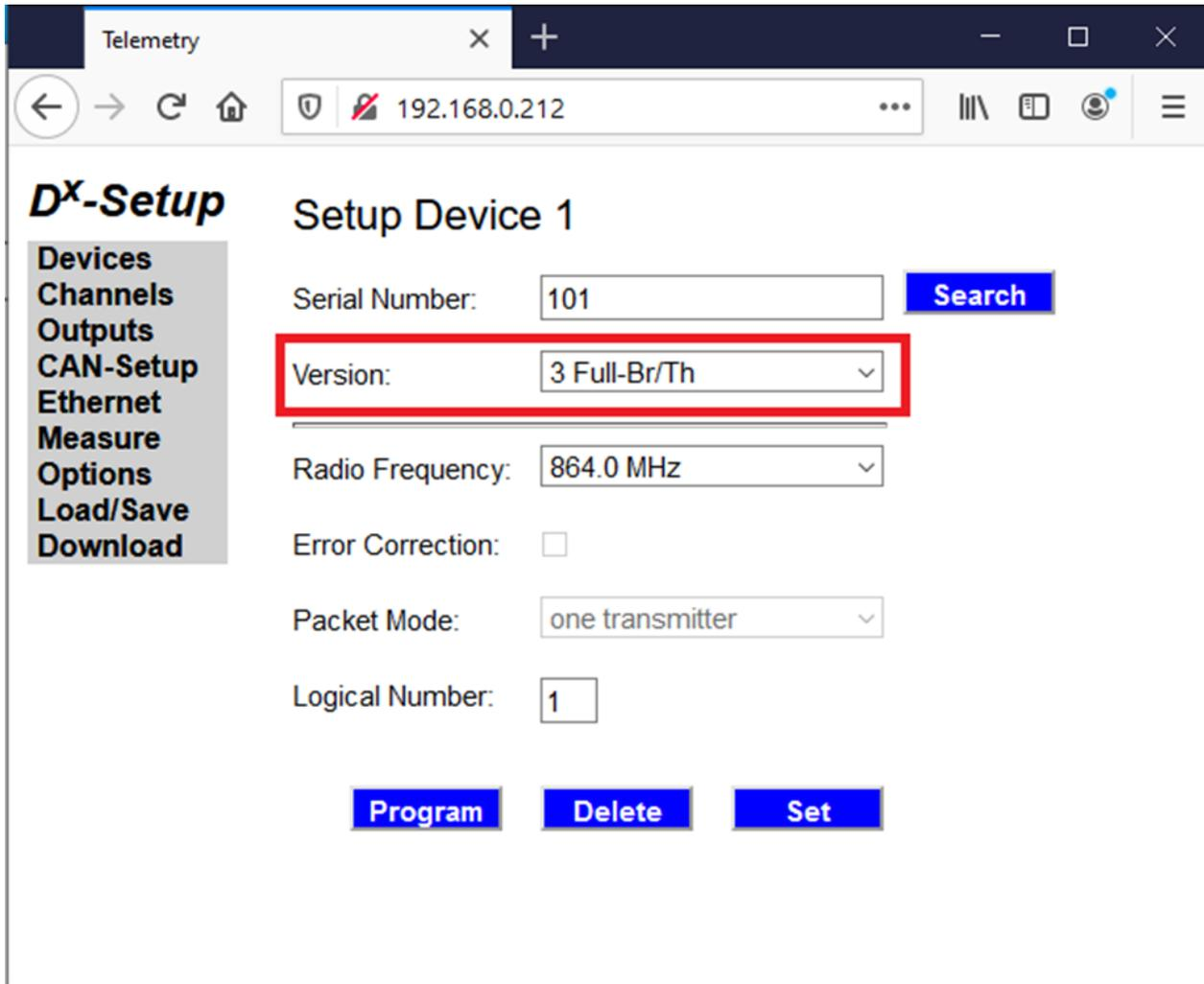
The screenshot shows a web browser window titled "Telemetry" with the address bar displaying "192.168.0.212". The main content area is titled "D<sup>X</sup>-Setup" and "Setup Device 1". On the left, there is a sidebar menu with the following items: Devices, Channels, Outputs, CAN-Setup, Ethernet, Measure, Options, Load/Save, and Download. The main configuration area includes the following fields and controls:
