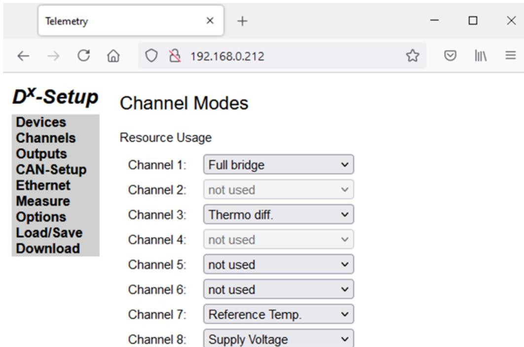
Fig. 68: Configuration menu channel mode
