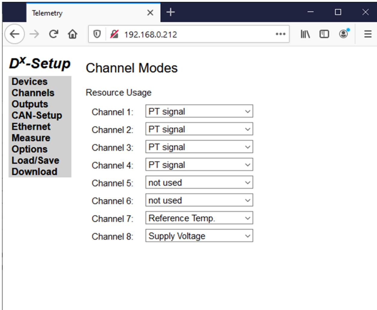
Fig. 86: Set channels to PT signal
