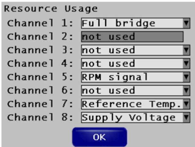
Fig. 108: Set Channel 1 to Full bridge, Channel 5 to RPM signal
