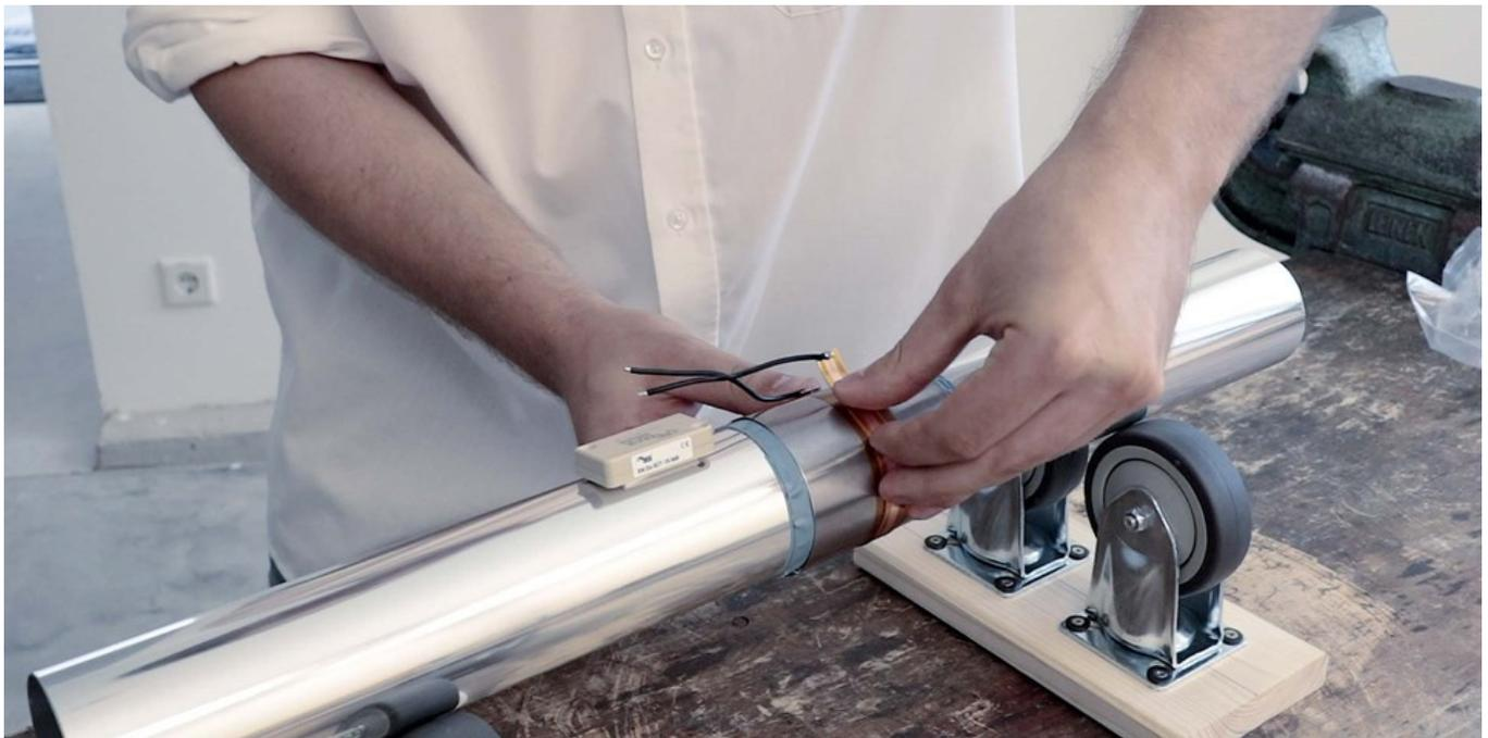
Fig. 39: Assembly of the secondary winding
