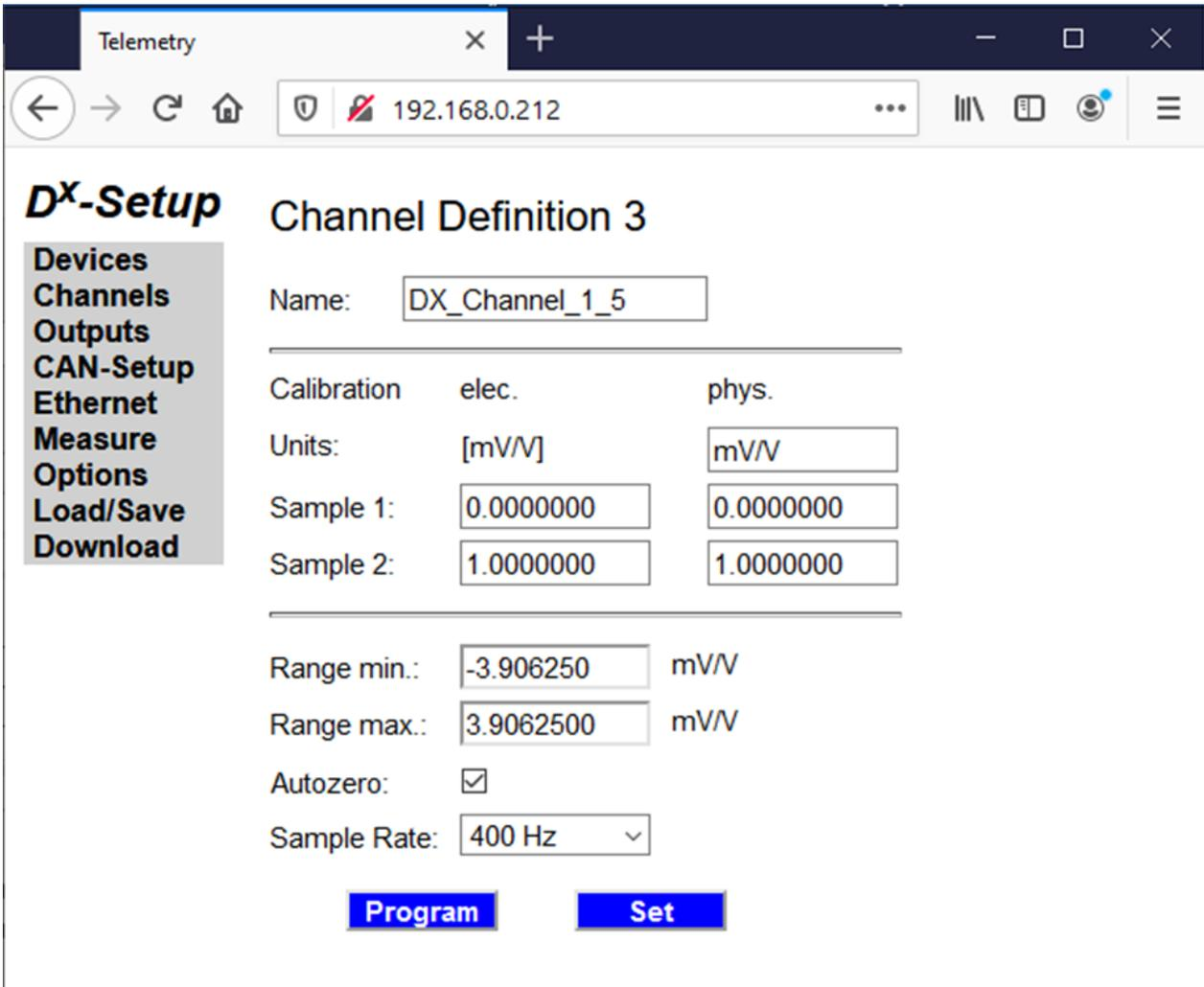
Fig. 78: Configuration menu for one full bridge
