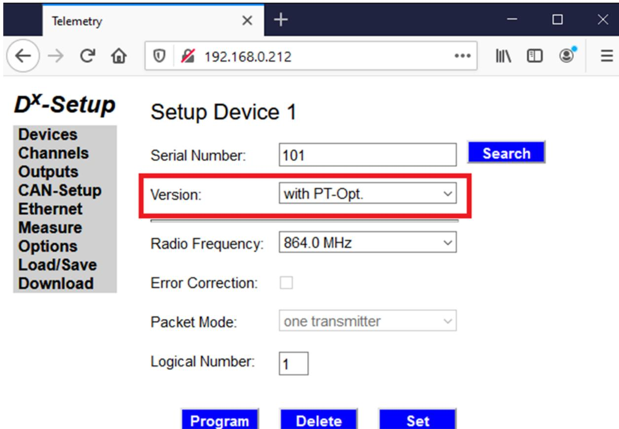
The screenshot shows a web browser window titled "Telemetry" with the address bar displaying "192.168.0.212". The main content area is titled "D<sup>X</sup>-Setup" and "Setup Device 1". On the left, there is a sidebar menu with the following items: Devices, Channels, Outputs, CAN-Setup, Ethernet, Measure, Options, Load/Save, and Download. The main configuration area includes the following fields and controls:
