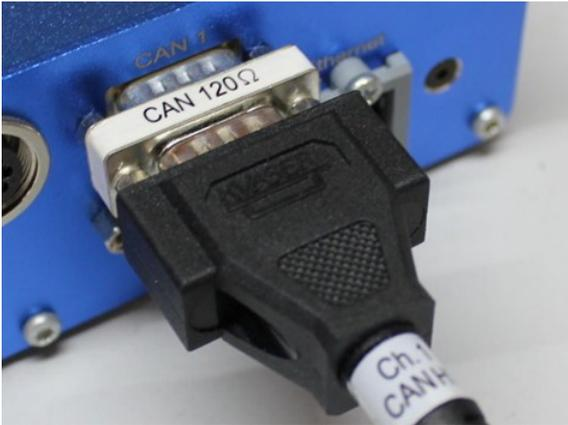
Fig. 58: Plugged CAN terminating resistor (120 Ω)
