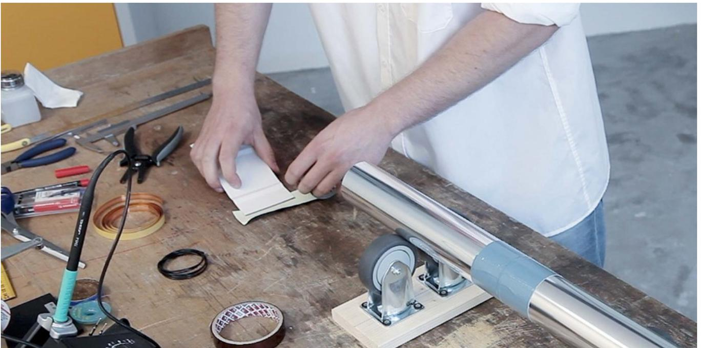
Fig. 26: Apply black isolating tape to one end of the Mu metal
