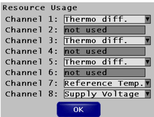
Fig. 114: Channel settings with 3 thermocouples
