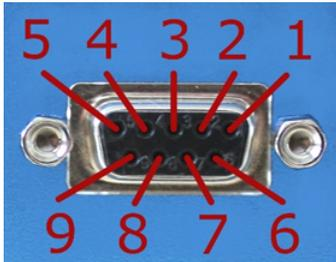
Fig. 15: Pin configuration DSUB-9 CAN socket
