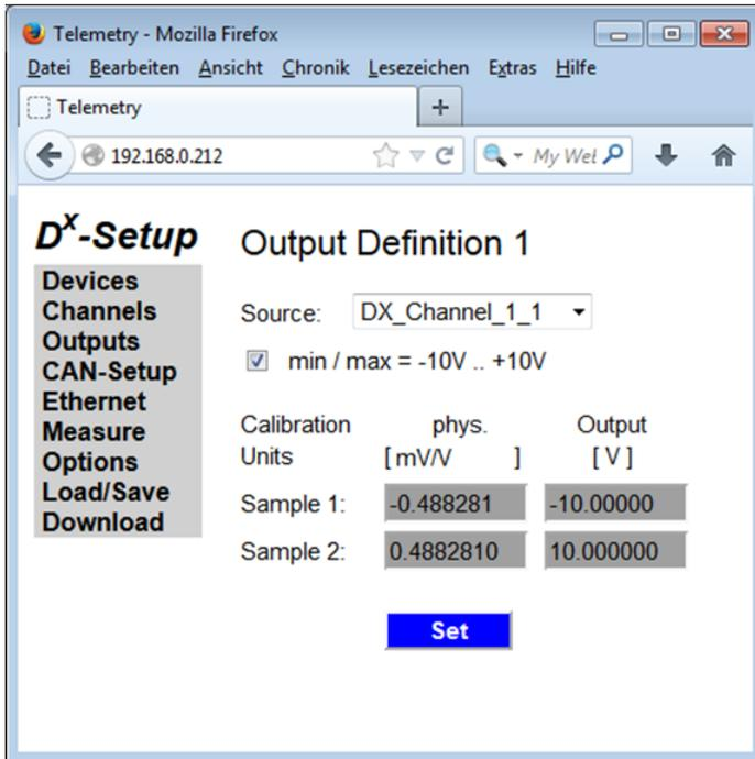
Fig. 96: Configuration menu analog output
