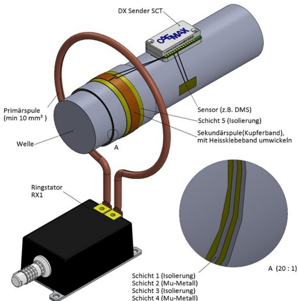
Fig. 24: Application ring stator
