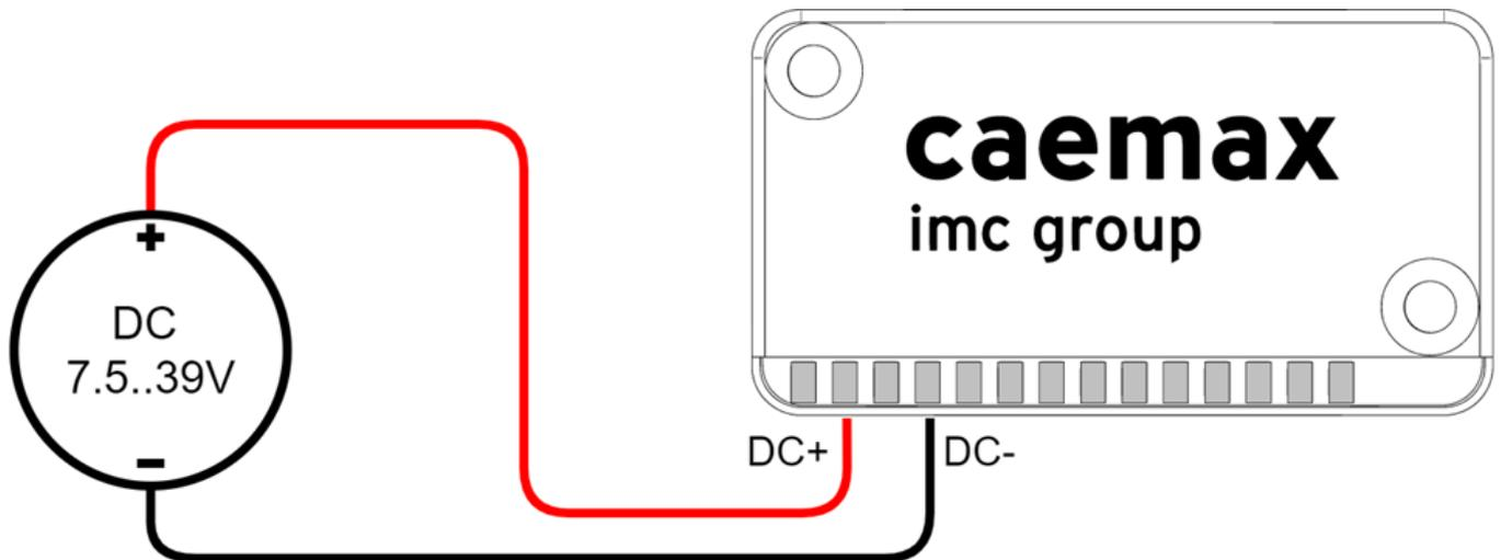
Fig. 10: Connection of D<sup>X</sup>-SCT to a DC voltage source
