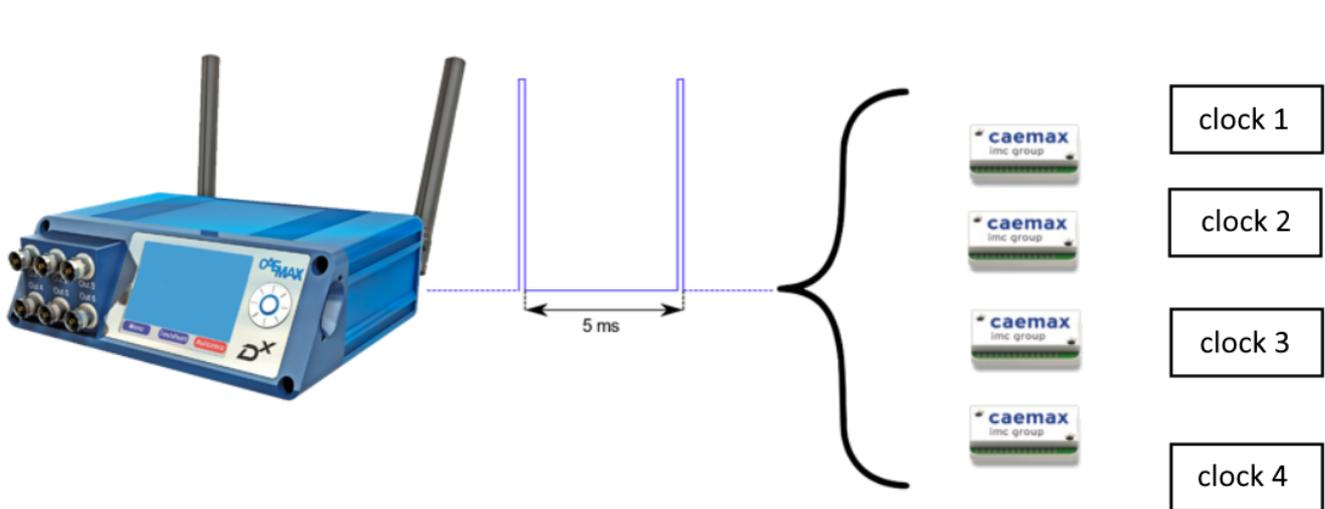
Fig. 16: Overview synchronization of multiple D<sup>x</sup>-SCTs
