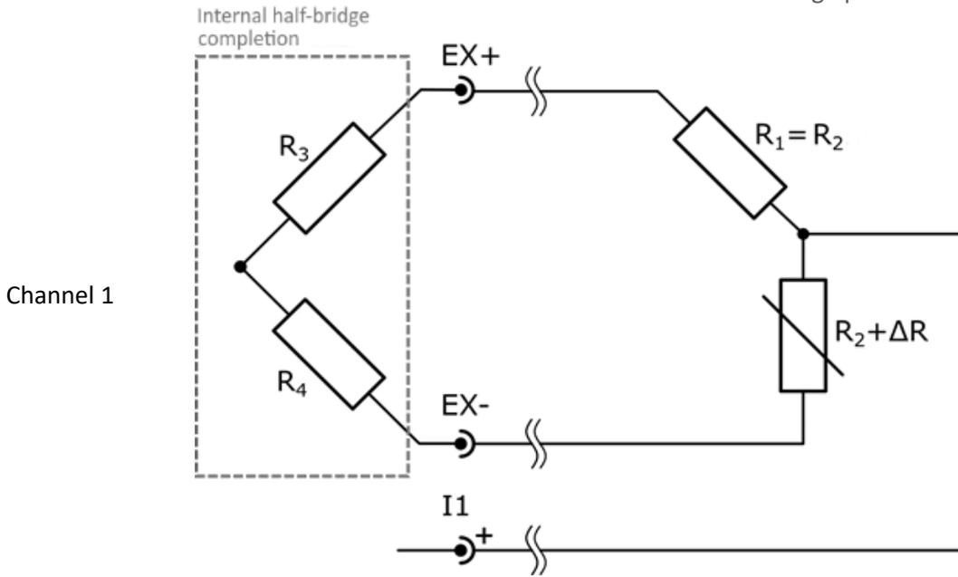
$R_1$ : Complementary resistor with high precision and stability
