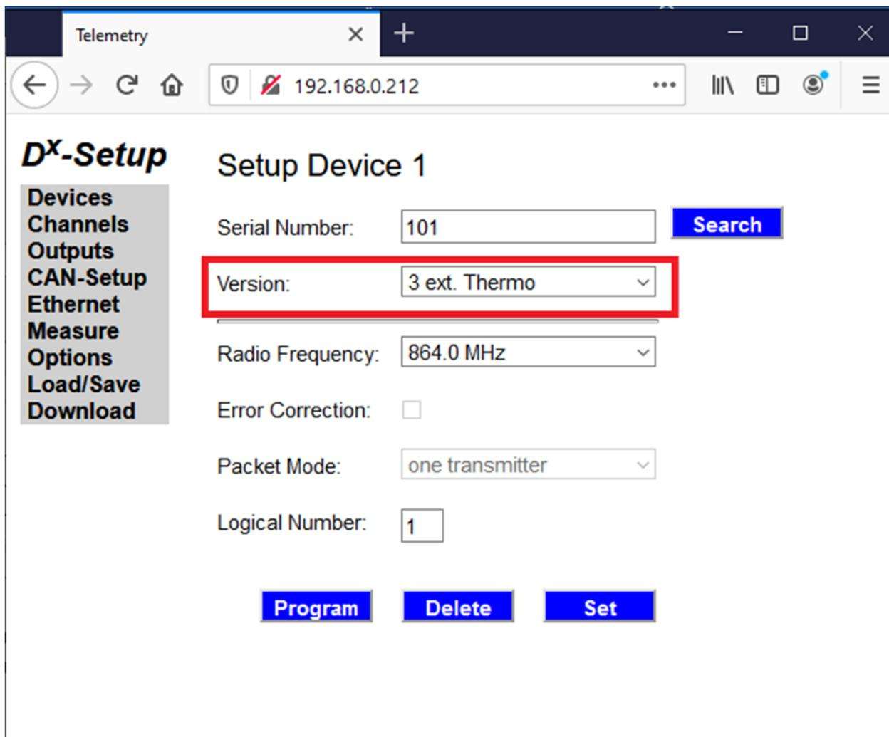
The screenshot shows a web browser window titled "Telemetry" with the address bar displaying "192.168.0.212". The main content area is titled "D<sup>x</sup>-Setup" and "Setup Device 1". On the left, there is a navigation menu with the following items: Devices, Channels, Outputs, CAN-Setup, Ethernet, Measure, Options, Load/Save, and Download. The main configuration area contains the following fields and controls:
