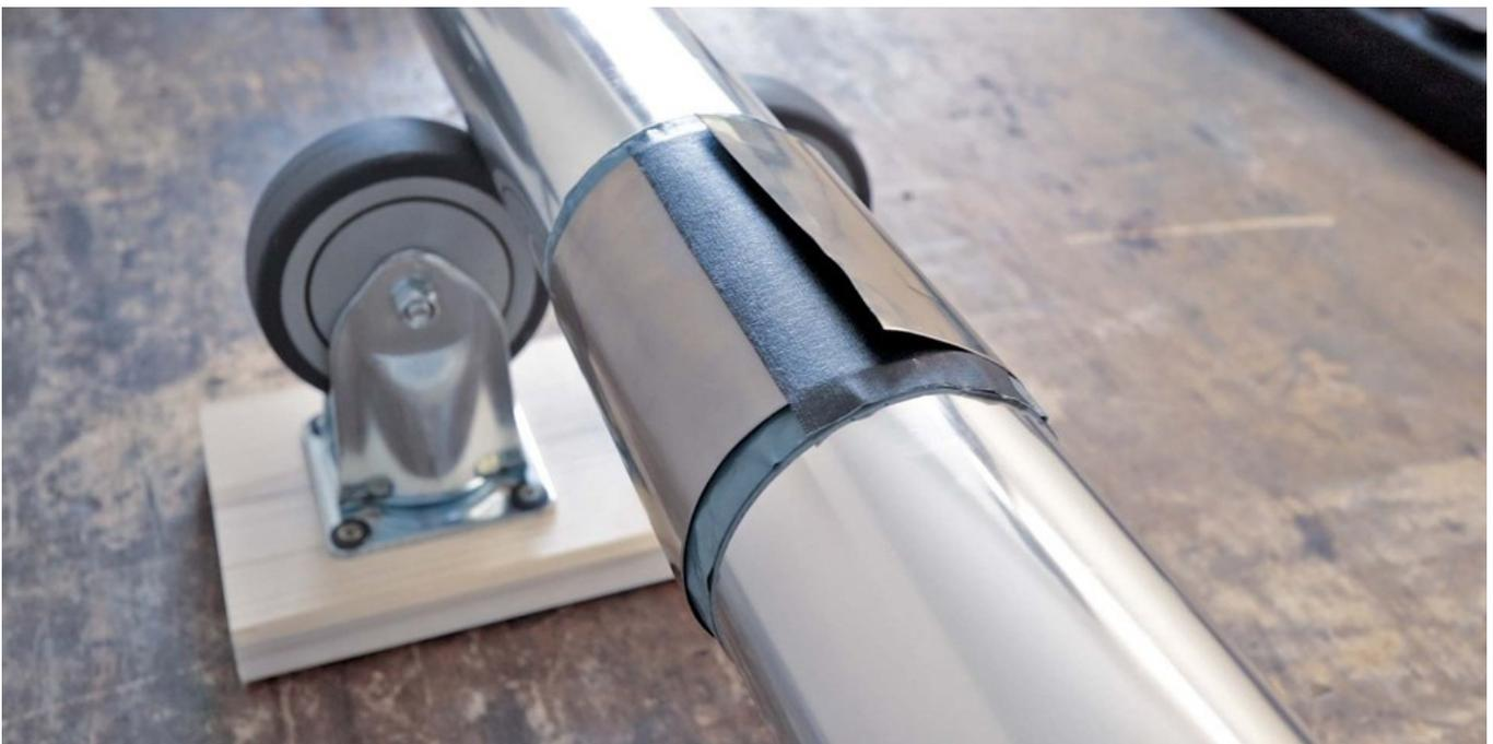
Fig. 32: After applying the second Mu metal layer
