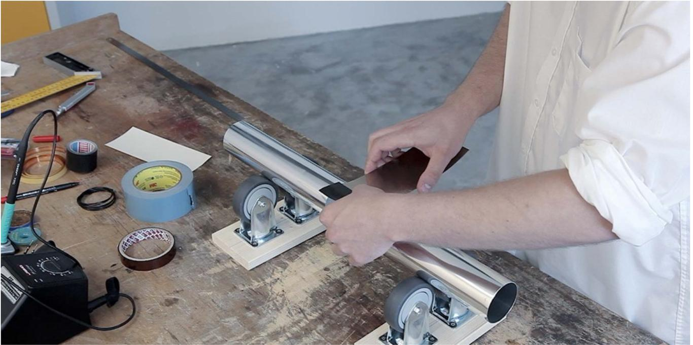
Fig. 31: Apply second Mu metal layer
