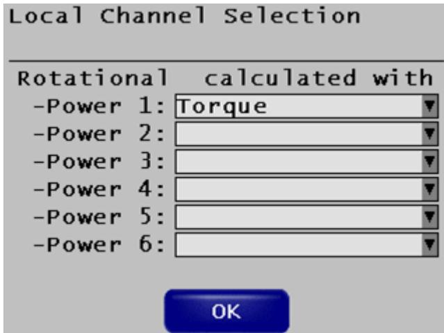
Fig. 110: Set Power 1 to the channel coupled with the torque
