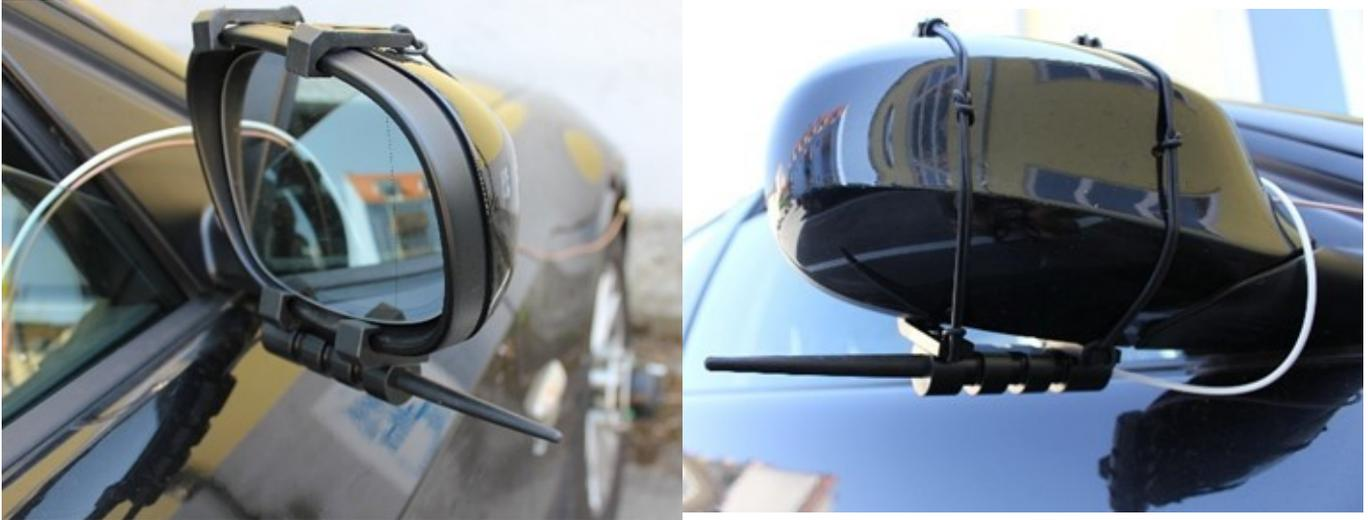
Fig. 117: D<sup>x</sup> side mirror antennas
