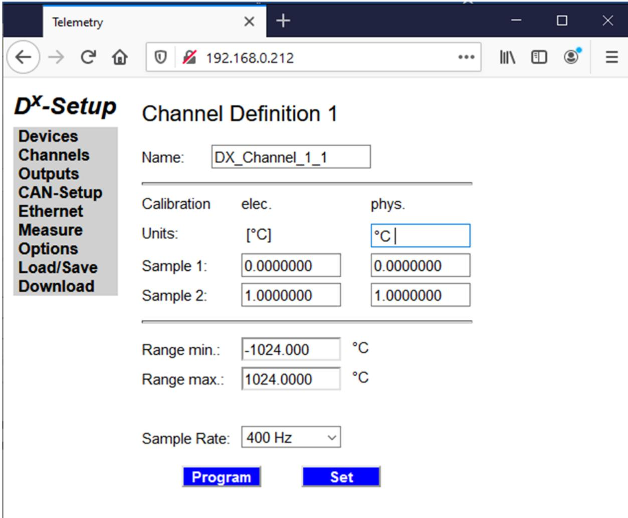
Fig. 87: Configuration menu for channels with Thermo signal
