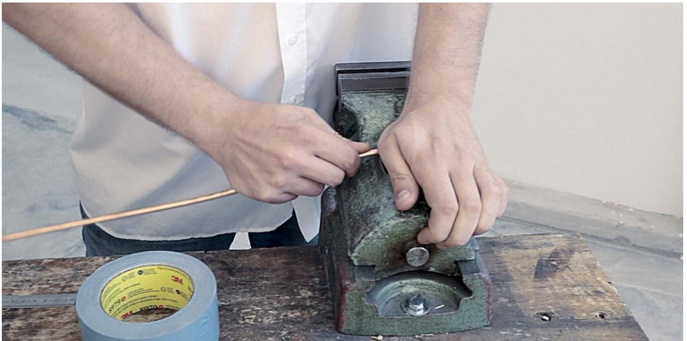
Fig. 46: Bend the ends of the copper wire
