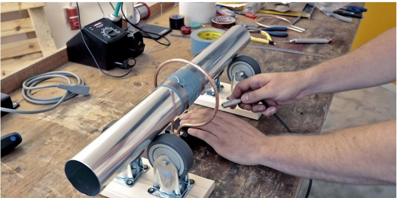
Fig. 54: Connect the power cable to the ring stator
