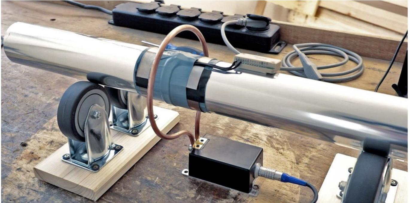
Fig. 55: Complete assembly: ring stator and secondary winding
