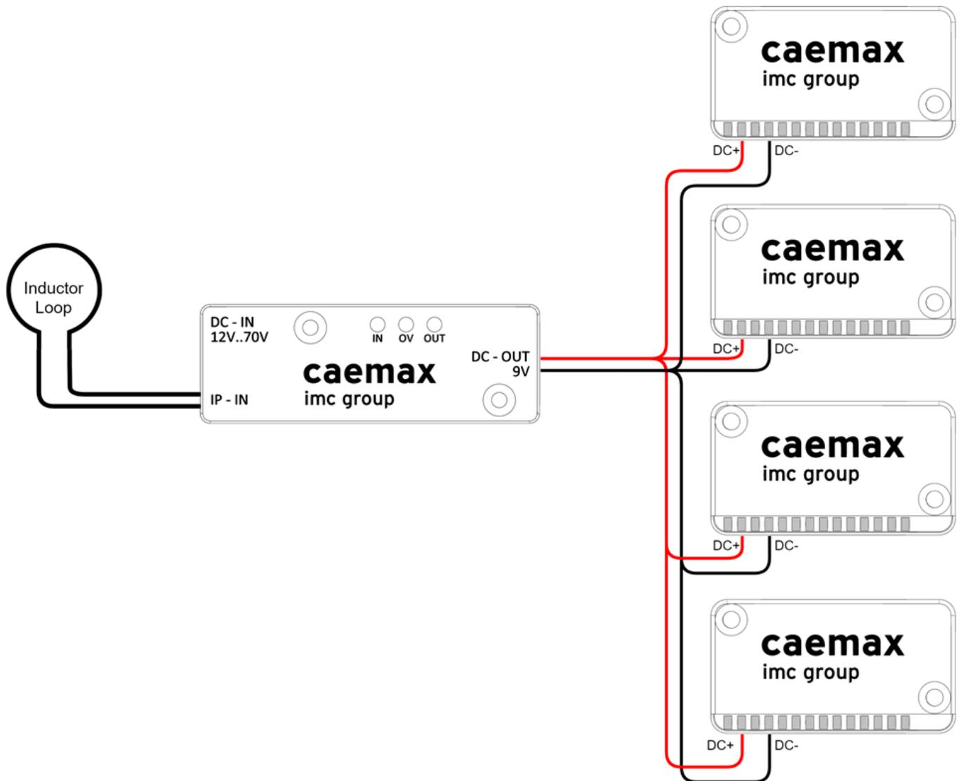
Fig. 21: Connection scheme of D<sup>x</sup>-OVP modules for one inductive source and 4 D<sup>x</sup>-SCT units
