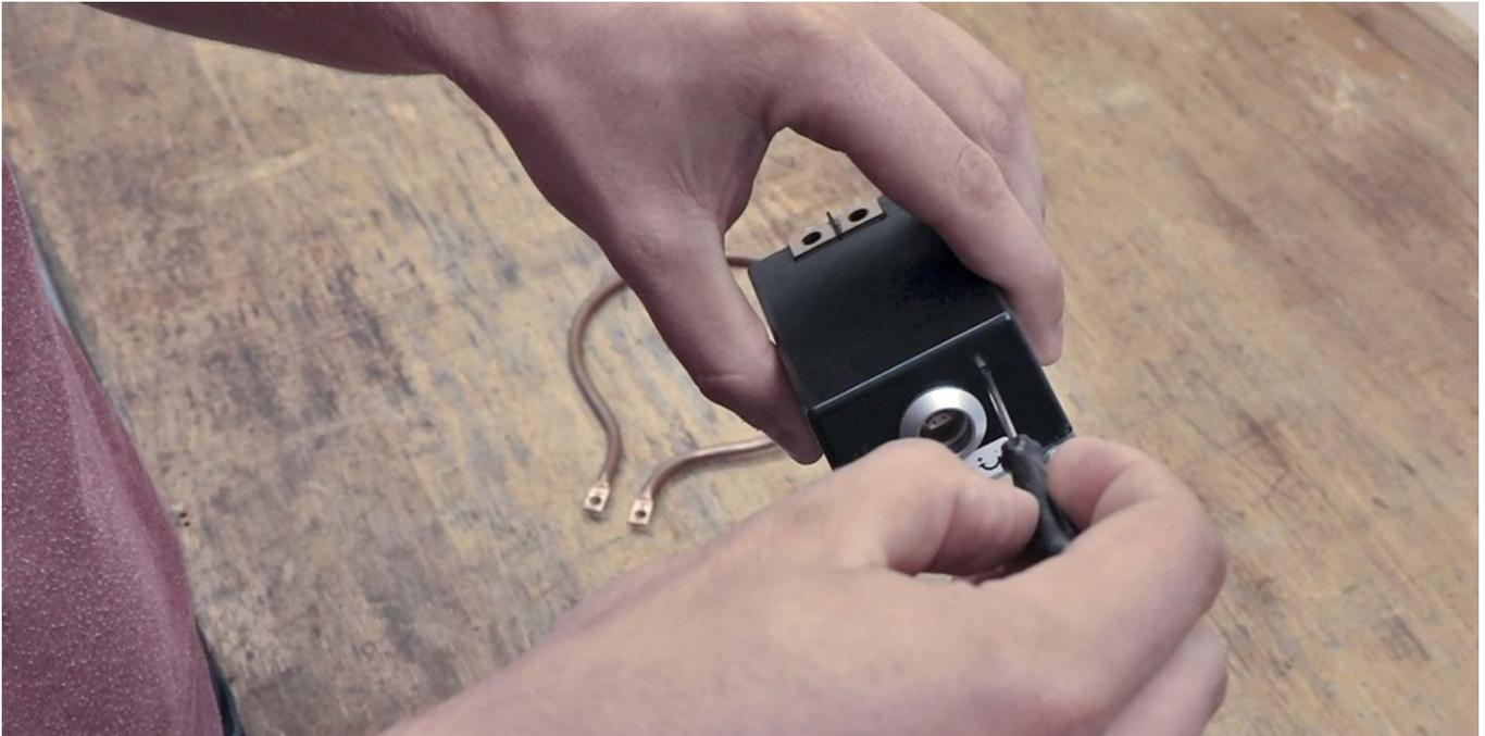
*Fig. 53: Set the voltage regulator to the minimum position*
