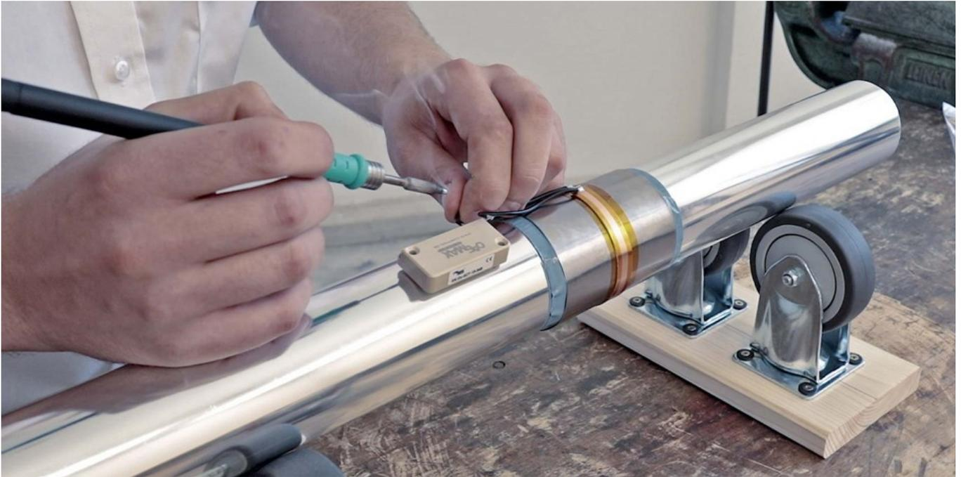
Fig. 40: Soldering the wire ends to the D<sup>X</sup>-SCT transmitter unit
