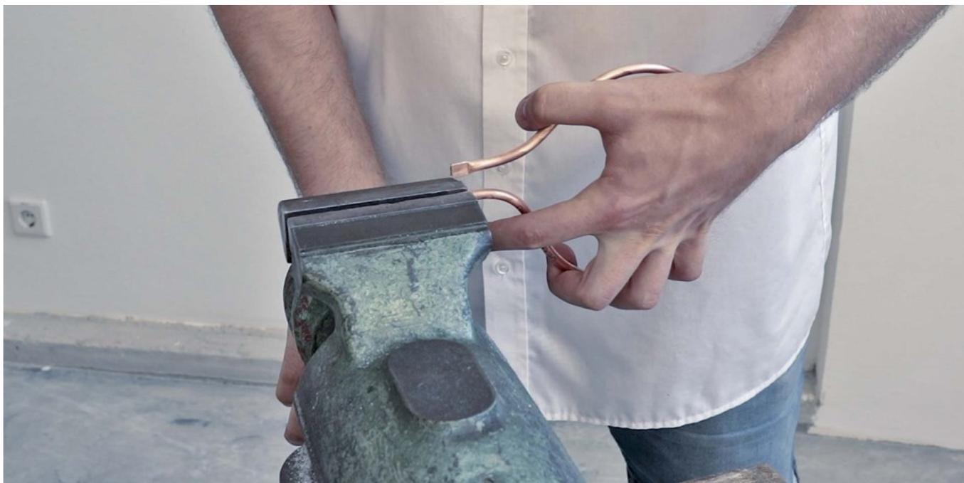
Fig. 48: Press the copper tube together at both ends
