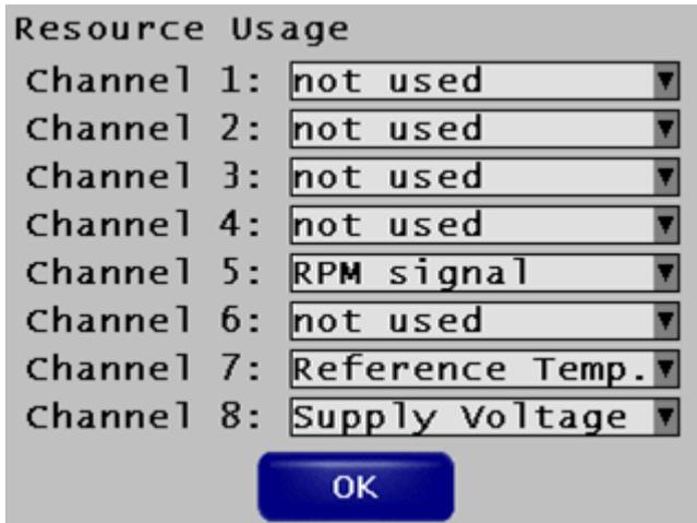
Fig. 106: Set channel 5 to RPM signal
