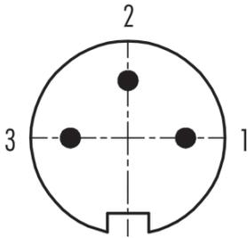
Fig. 14: Pin configuration power socket Binder M16 (3-pin)
