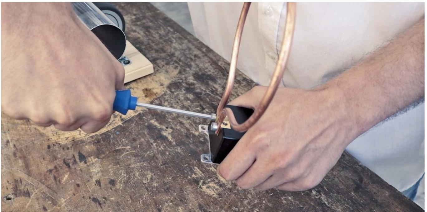
Fig. 52: Screw primary winding to ring stator
