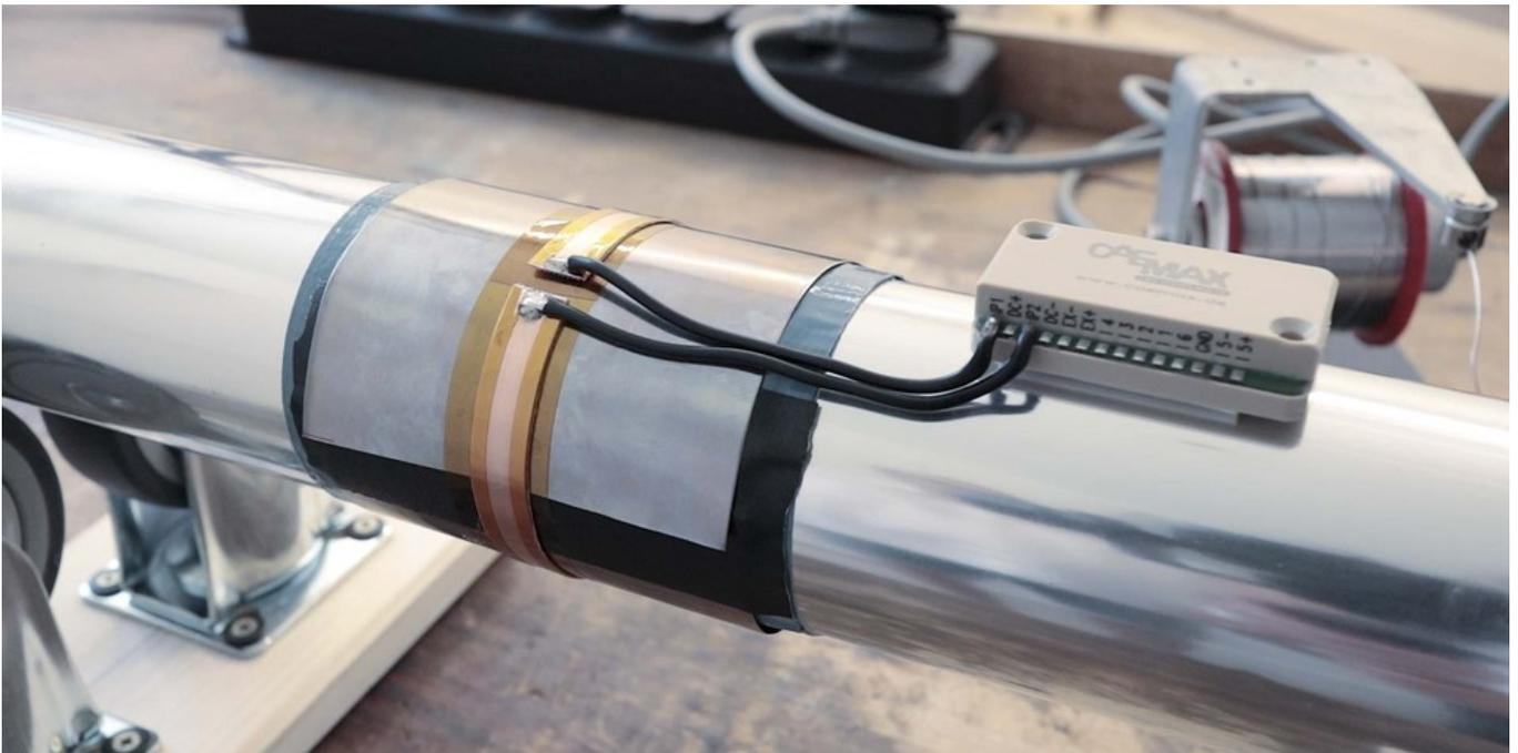
Fig. 41: Secondary winding connected to transmitter unit D<sup>X</sup>-SCT
