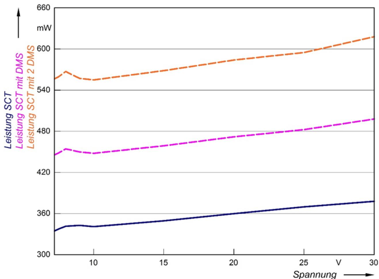
Fig. 17: Power consumption of the D<sup>x</sup>-SCT power consumption SCT with 2 strain gauge out of the measurement setup SCT and power consumption SCT with DMS
