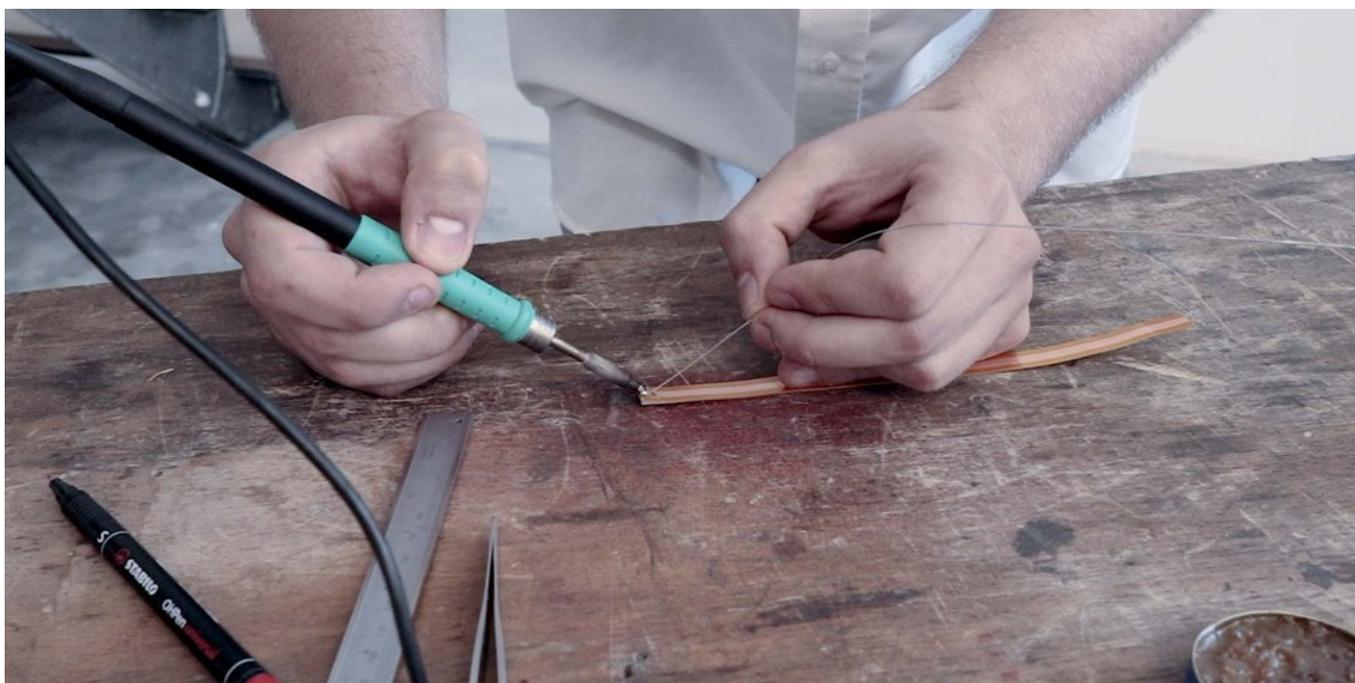
Fig. 36: Tin both ends of the copper strip
