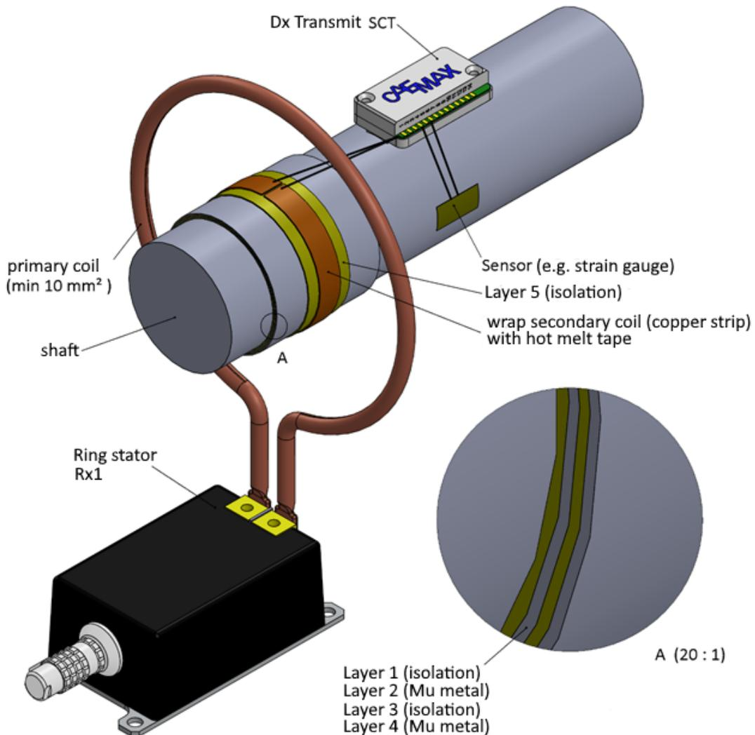
Fig. 18: Overview: installation of the Ring stator
