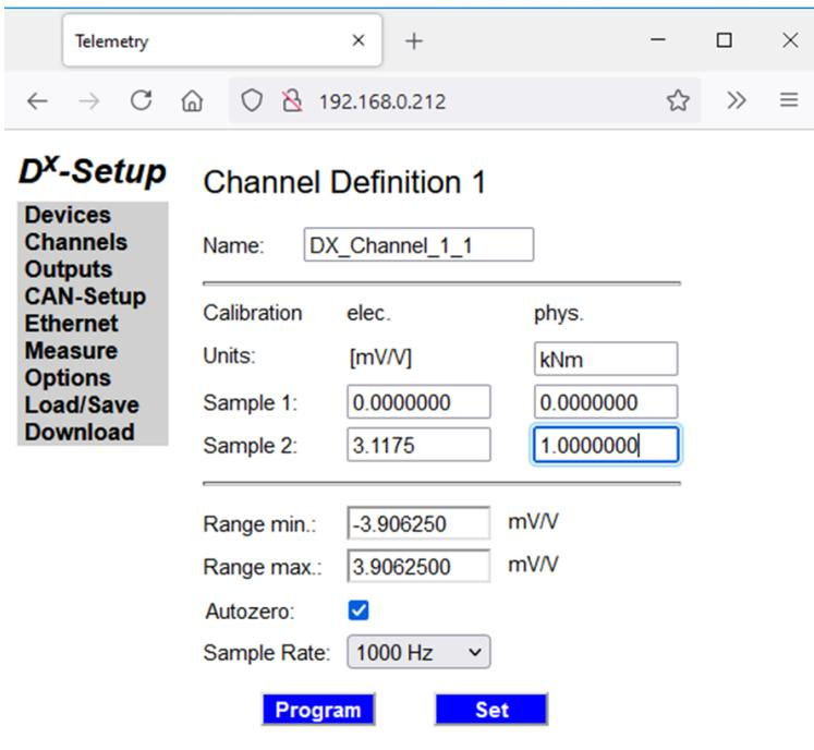
Fig. 72: Example of sensitivity (from the calibration record)
