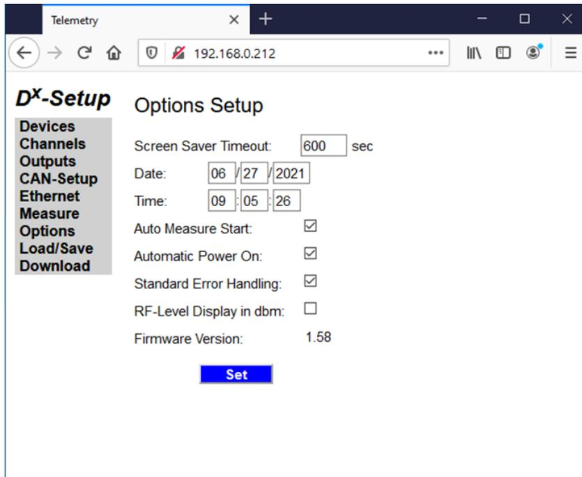
Fig. 103: Options menu / Start measurement automatically
