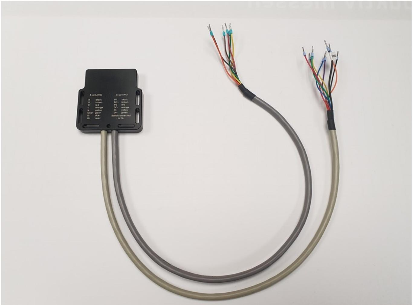
Fig. 7: DX-SCT with connection cable integrated in a special housing
