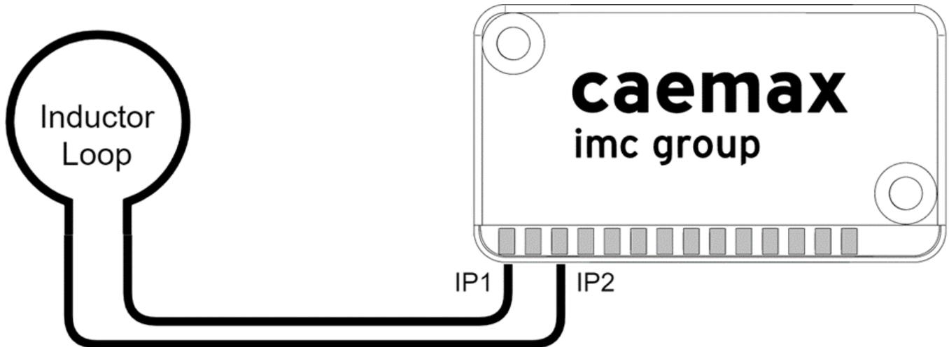
Fig. 11: Connection of D<sup>X</sup>-SCT to an inductive voltage source
