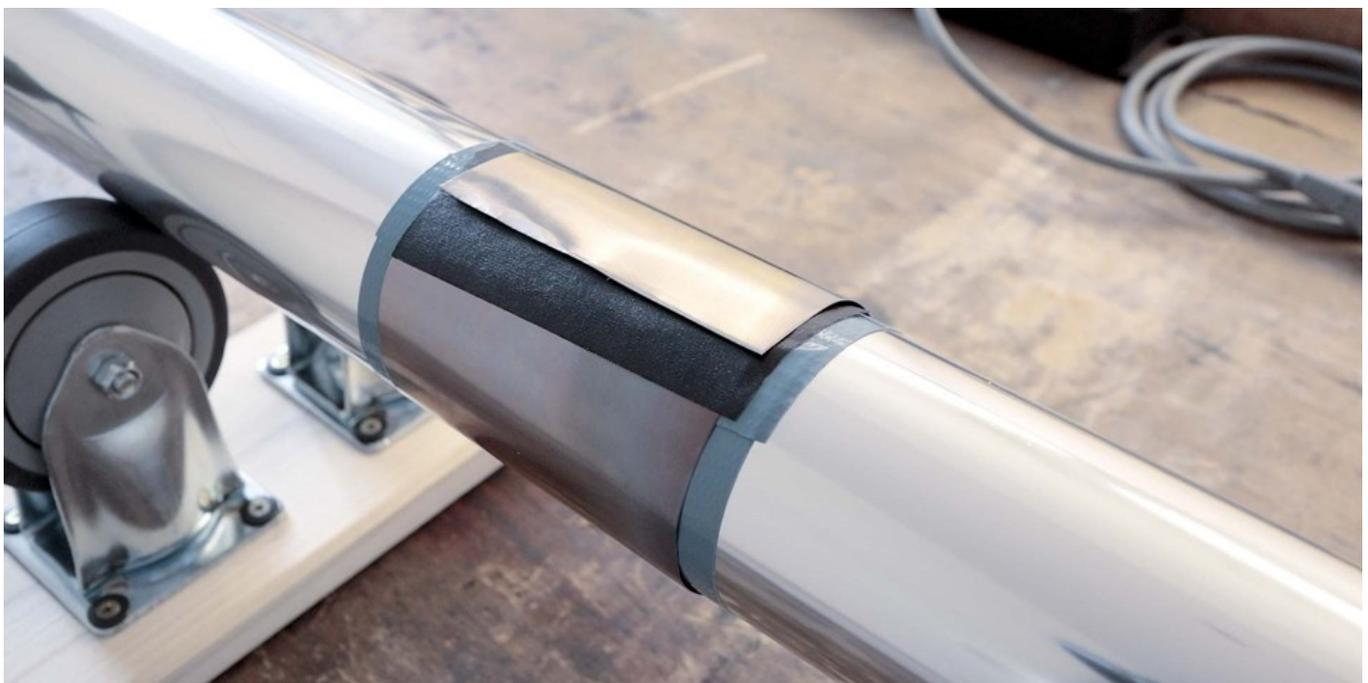
Fig. 28: After applying the first mu-metal layer
