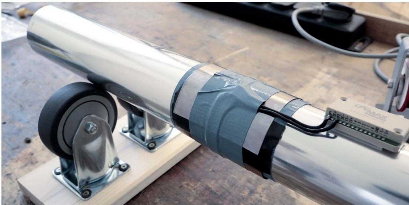
Fig. 43: The finished secondary winding
