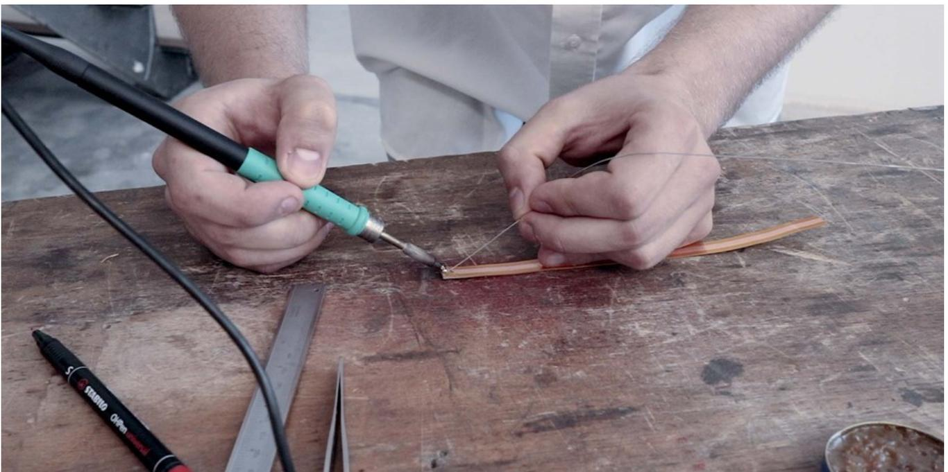
*Fig. 38: Solder the wires for the inductive power supply to the copper strip.*
