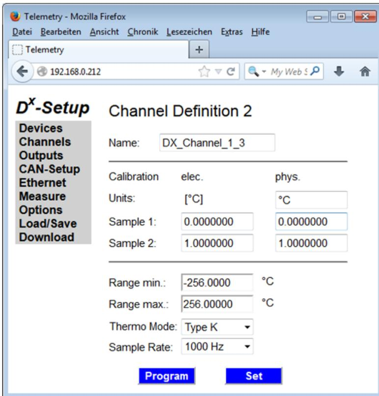
Fig. 74: Configuration menu thermocouple
